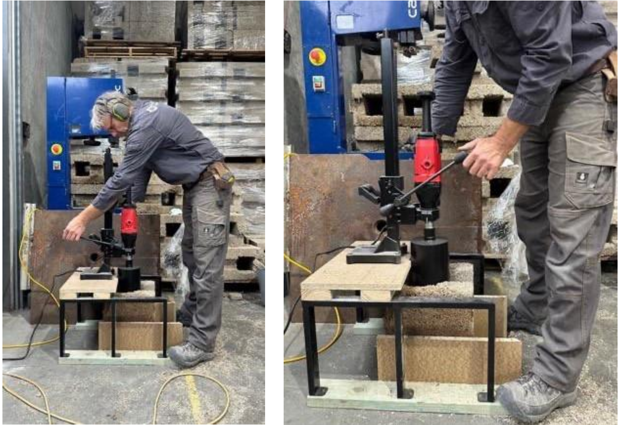
Figure 34 - Cutting a hole with a concrete hole saw
