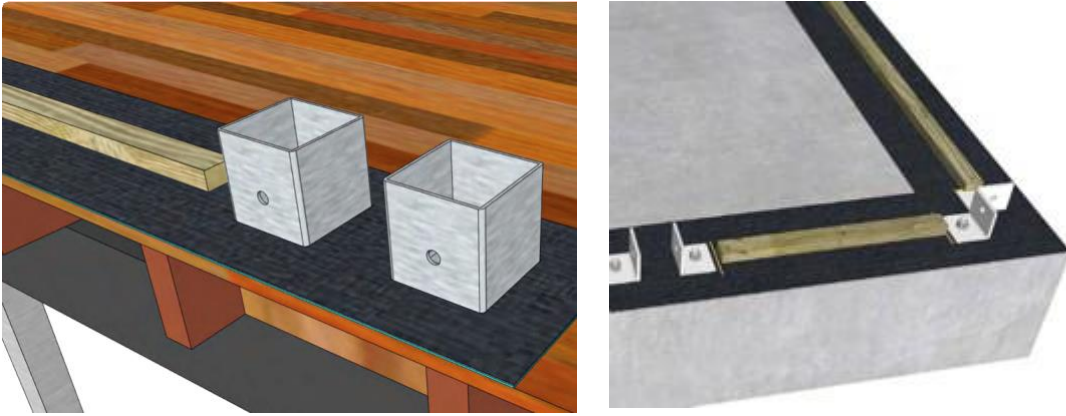
Figure 27 - Steel foot (stanchion) installation
