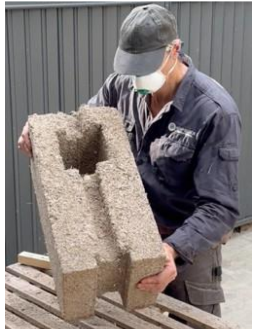
Figure 36 - Creating a tongue groove
