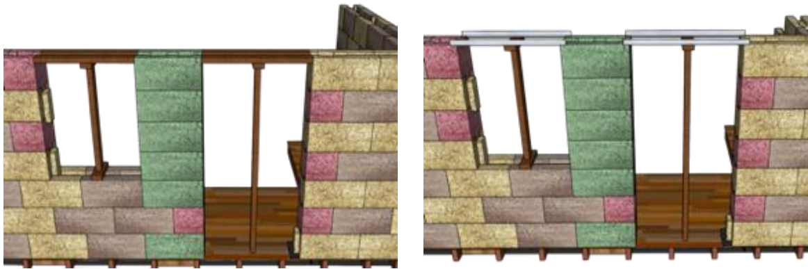
Figure 68 - Installing temporary supports
