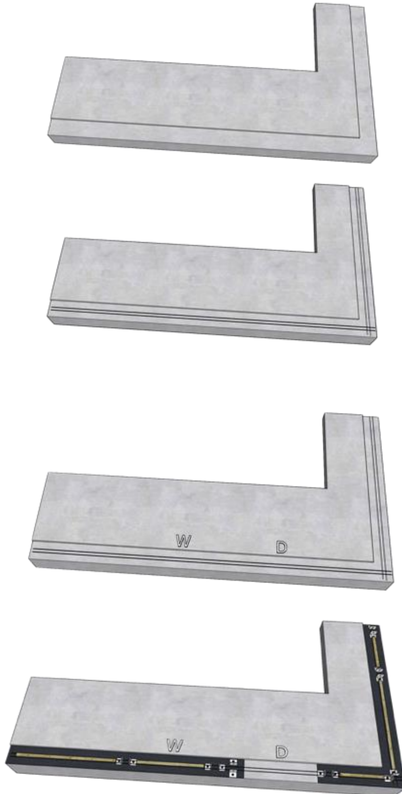
Figure 22 - Marking out walls and column positions
