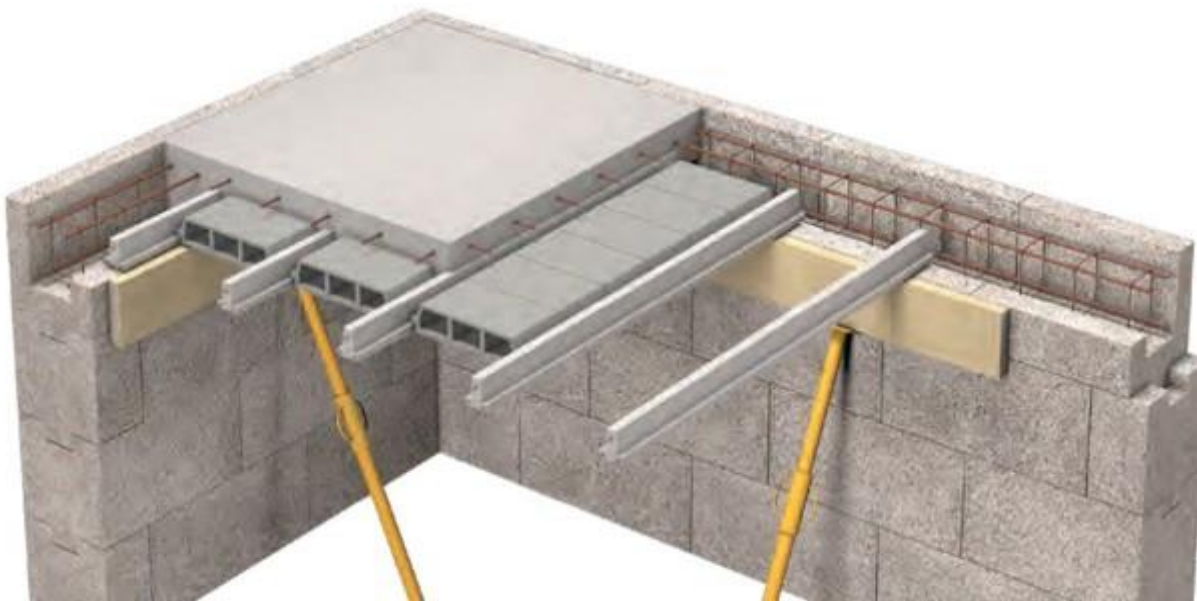
Figure 101 - Casting a concrete second floor system
