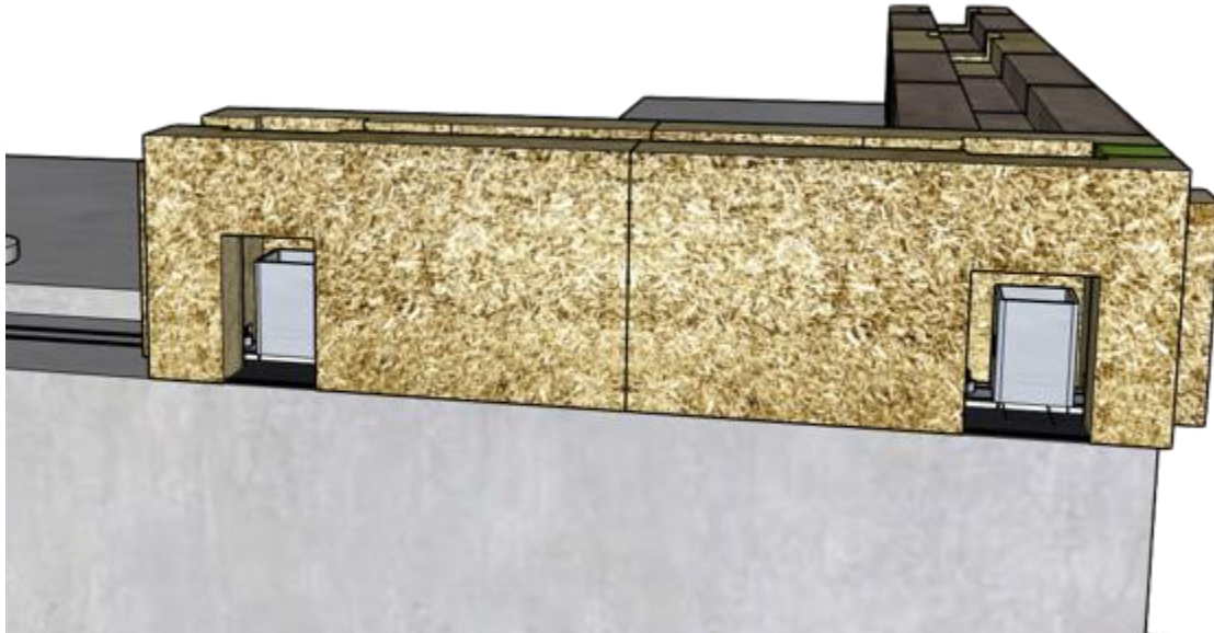
Figure 39 - Cutting out access holes
