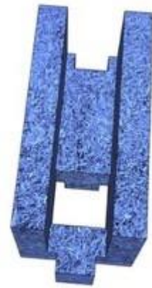
Figure 94 - Column cut out of a U block
