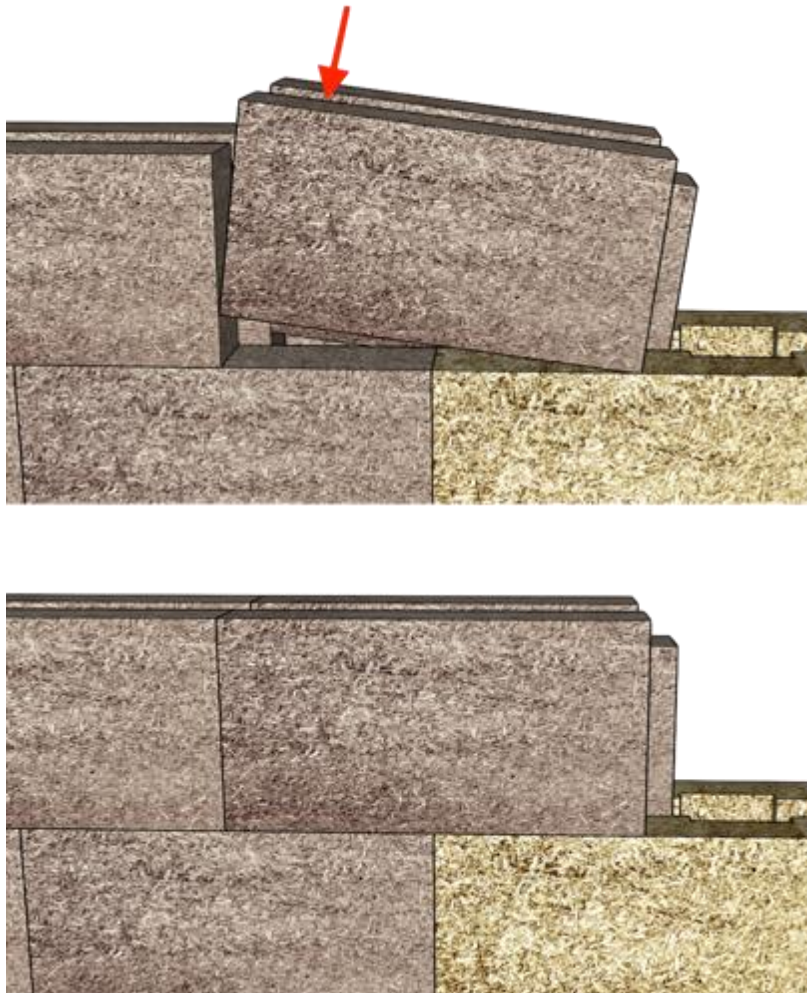
Figure 47 - Interlocking the tongue and groove blocks
