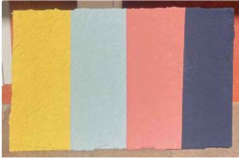
Figure 114 - Sample chalk paint colours on a lime rendered fibre-cement backing
