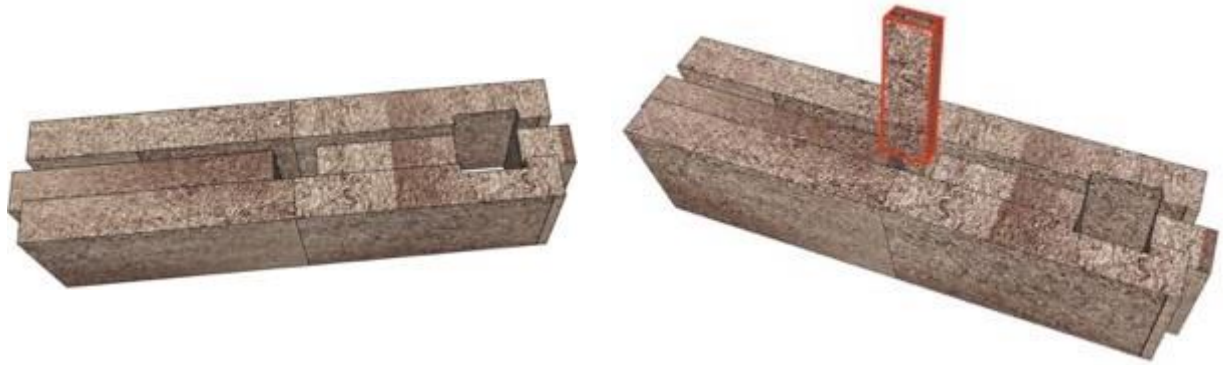
Figure 40 - Filling the void at two grooves
