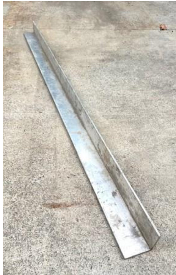
Figure 67 - Aluminum support angle
