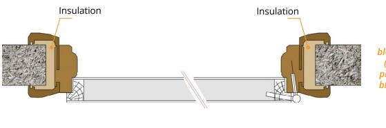
Beware of securing blocks above the opening (propped, with a lintel plus a board to keep the blocks above in line with the rest of the wall.
